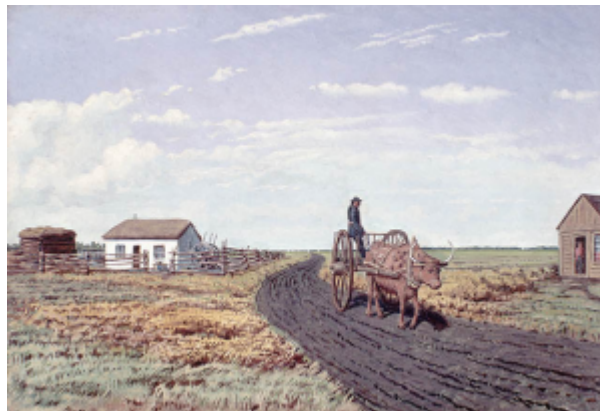
Figure 8.17 Red River carts were amphibious craft consisting of a flatbed attached to two large, convex spoked wheels. No metal was used in their construction and the wheels could be removed and strapped to the bottom so that the vehicle became a raft. They were invariably pulled by oxen. (Painting by William Hind, ca. 1862)
