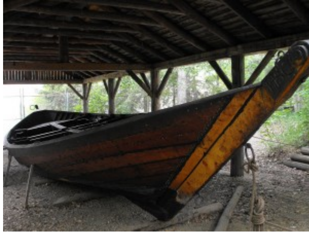
Figure 14.10 The York boat (on which the York/Columbia Express depended) is descended from the yole, a type of fishing boat found in the Orkney Islands, from where many HBC servants came. The yole, for its part, is descended from Viking boat design. The York boat has elements of design continuity that stretch back from the 19th century to the time of Vinland and earlier.
